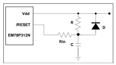
Fig. 5-34 External Power-Up Reset Circuit
